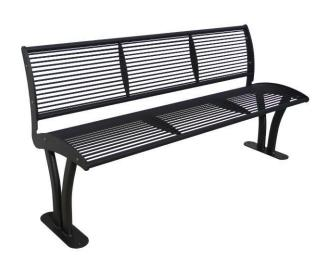
Bench Tauri is composed of two lateral supports made of laser-cut flanges, to which are welded two oval tubulars sec. 60x30 mm serving as legs and an oval base plate 360x100 mm.
